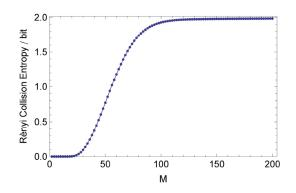
Figure 8. Example of the Conditional Rényi collision entropy of order two for bits being transmitted with  $\langle n \rangle = 100/\text{bit}$  signal as a function of the number of bases M.
