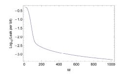
Figure 6. Logarithm of the loss per bit to Eve,  $t_{\rm bit}$ , as given by the POVM calculation that provides  $P_e$ . Here  $\langle n \rangle = 1000$ .
