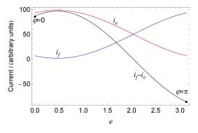
Figure 7. Photon currents  $i_e$  and  $i_f$  obtained from the pin diodes and the final difference current  $\Delta i = i_f - i_e$  as a function of the input phase  $\phi$ . Particular values are indicated with  $\phi = 0$  and  $\phi = \pi$  that represent bits 0 and 1.
