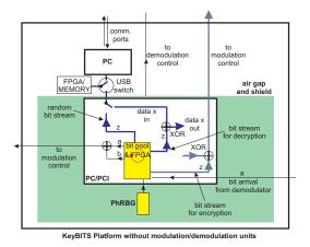
Figure 5. KeyBITS modular secure communications platform. See Fig. 2 for more details.
